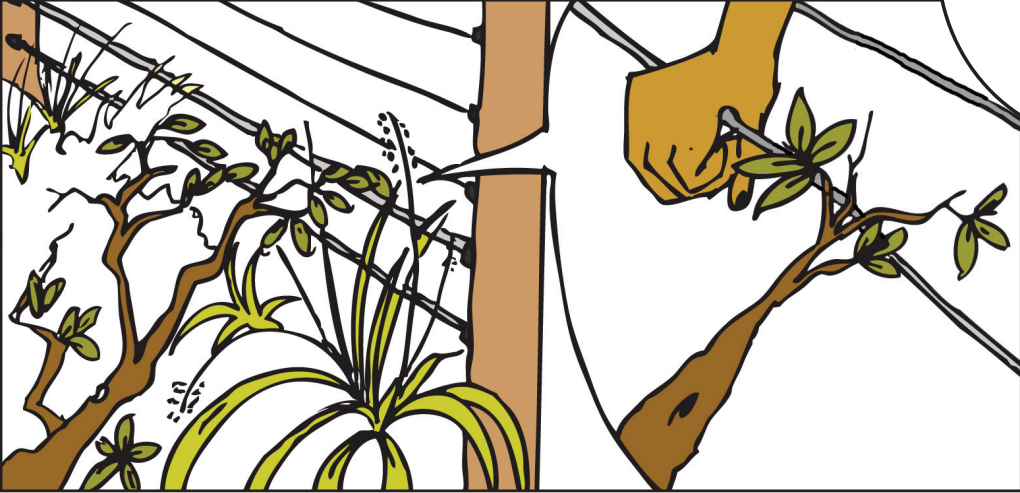
Fence loses power (shorts) if vegetation touches the live wire
